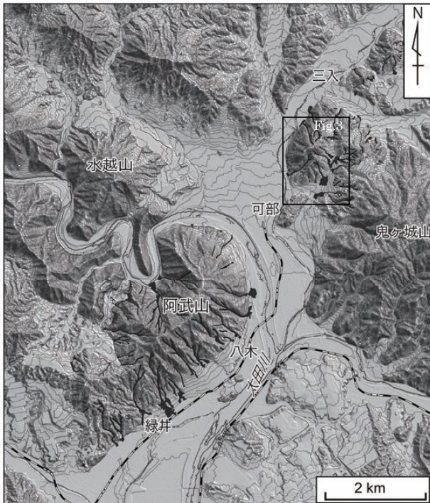
Fig. 2 Map shows the distribution of debris flows by heavy rainfall at Hiroshima on August 19 - 20, 2014. Black shapes indicate debris flows (from GSI, 2014 2 ).
